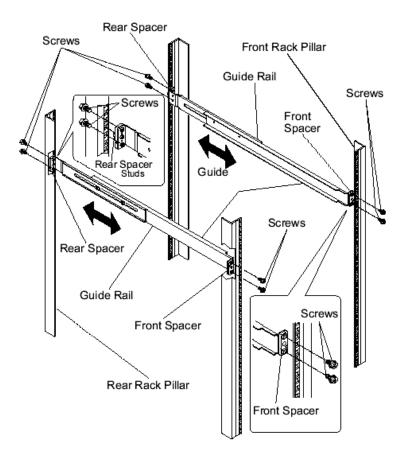
Installing the Guide Rails diagram
