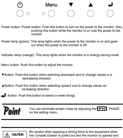
being used, as there is a risk that the rack may fall over. Do not strongly press on the monitor's screen, scratch it with sharp objects or place magnetic objects near it. Doing so may damage the monitor.
