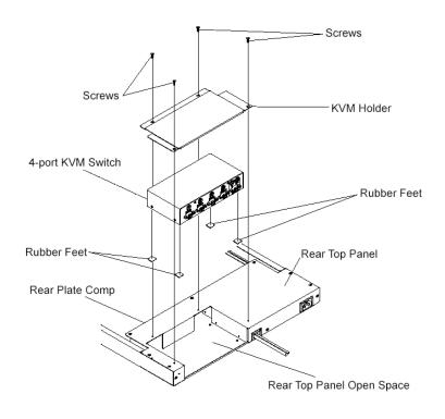
Installation Method 1: 4-port KVM switch Assembly Diagram (viewed from the left rear)
