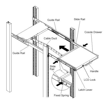
Inserting the slide module diagram
