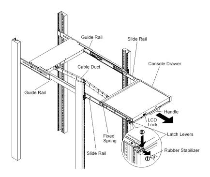
Pulling out the slide module diagram
