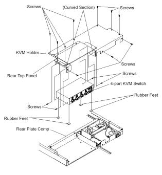
Installation Method 3: 4-port KVM switch Assembly Diagram (viewed from the left rear)
