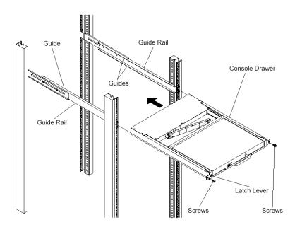
Installing the Console Drawer diagram
