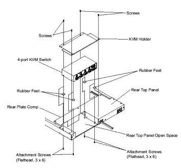
Installation Method 2: 4-port KVM switch Assembly Diagram (viewed from the left rear)
